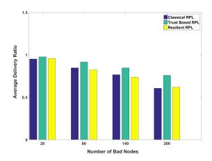
Figure 8: Average delivery ratio versus number of bad nodes (the more the better)
