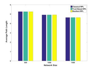
Figure 4: Average path length versus network size (the less the better)
