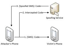
Figure 2: Theoretical exploit approach against XMS and JaxtrSMS
